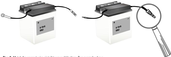
Step 2: Match the correct wire pigtail to your old battery. See example above
