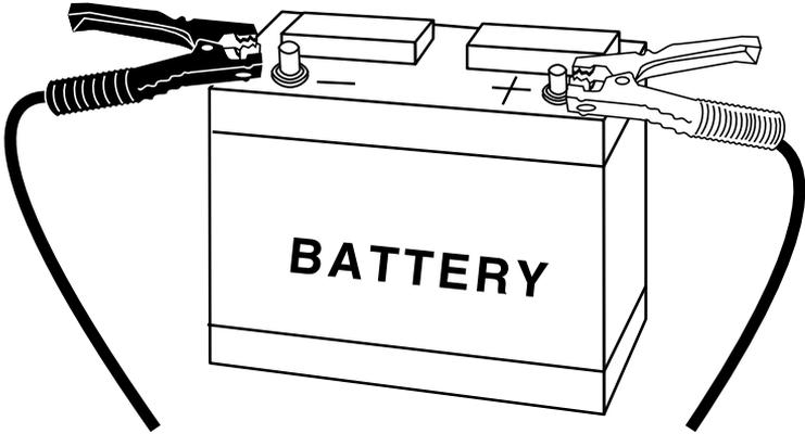
2. Connect to only one 6-volt or 12-volt battery at a time.
