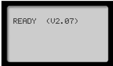
The program can be updated to the most recent version by reflashing the memory. Before turning the unit on hold the (N Exc.) and the (Y Enter) key down simultaneously. The following will appear.
