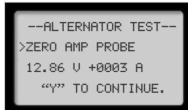
You will first be asked to zero out the Probe. Pressing the "Zero Amp Probe" on the keypad. Instead of +00003 A, it should read +00000 A.
