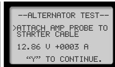
You will then be asked to attach the probe to a particular wire such as alternator output or starter cable.
