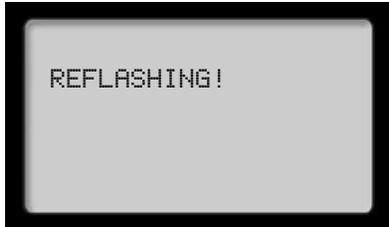
When a computer can be attached to the unit in the same way the test data can be downloaded. "REFLASHING!" will then appear while the program is updating.
