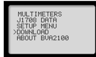
Using Auto Meter's optional adapter cord AC-10 insert the plug into the jack on the BVA-2100 and then plug the serial adapter into a free serial port on your computer.
