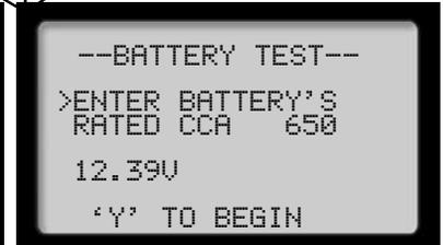
Using the (+) or (-) key adjust the CCA of the battery. Press (Y Enter) to begin test.
