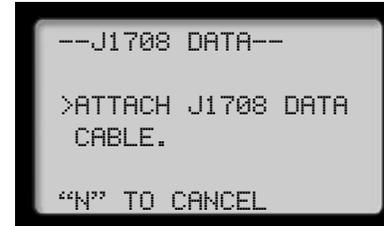
Attach the Optional **J1708 Data Cable**. If the cable is not correctly attached the test will not continue. Check the connection at the tester and the vehicle.
