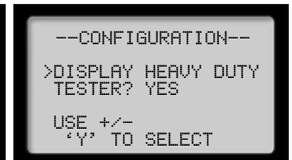
To configure for Heavy Duty select YES. Using the (UP) or (Down) key to select NO will give you a different main menu. The tester must be turned off and rebooted to include and changes. The two menus are listed below.
