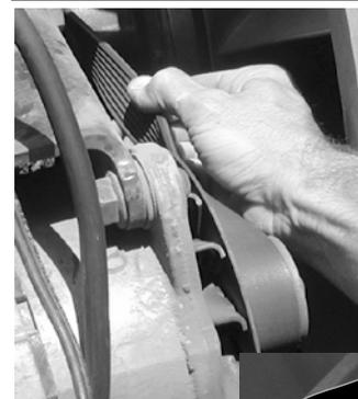
If the unit is setup to require visual checks you will be asked to inspect belt condition and tension. Also, if this is an individual alternator test and not part of the CHARGING SYSTEM test you will be asked to enter the alternator rating
